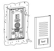
With help of a plain screwdriver, fix the aluminium front with especified screws, as shown on the picture.
