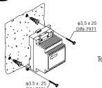
The power supply must be installed in a dry and protected place. It's recommended to protect the power supply by using a thermo-magnetic circuit breaker.
