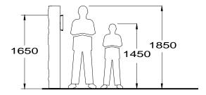
The upper part of the door panel should be placed at 1,65m. The surface door panel dimensions are the next:
